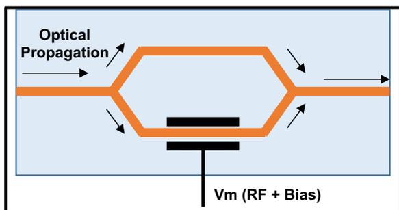
Fig. 3. A Mach-Zehnder modulator showing a diffused optical waveguide on LiNbO3 substrate. The group delay in the lower leg increases in proportion to an applied microwave field.
