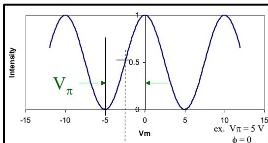
Fig. 4. The raised cosine intensity characteristic as a function of applied field. Linear small signal modulation is possible when the modulator is biased at  $V_\pi/2$ .
