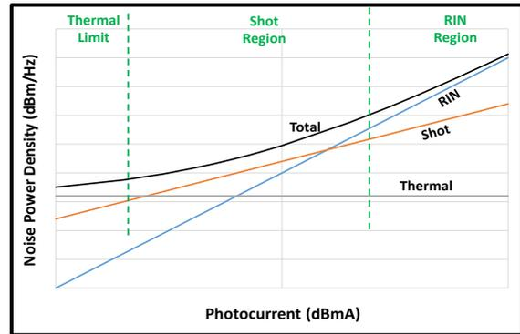
Fig. 6. Noise power at the output of a microwave link is dependent upon the detected photocurrent. 3 regions of operation result: thermal, shot, and RIN.
