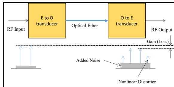
Fig. 5. A microwave link can be characterized by its gain (or loss), its added noise, and its nonlinear distortion.
