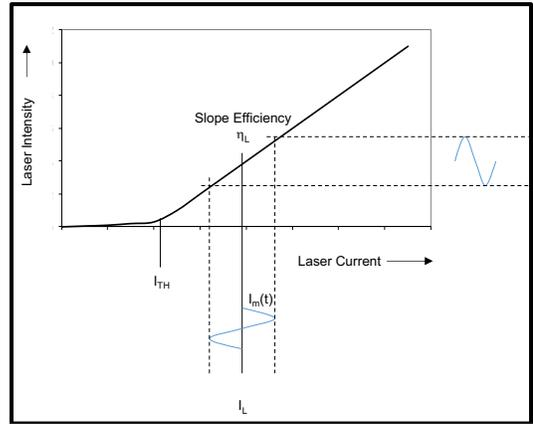
Fig. 2. Intensity directly modulated by microwave current.
