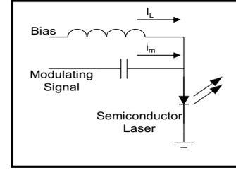
Fig. 1. Direct modulation: microwave current  $i_m(t)$  is coupled directly into a laser diode, along with the bias current  $I_L$ .
