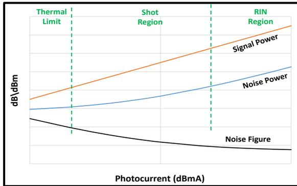
Fig. 7. Both noise and signal increase with the same 2:1 slope in the RIN region, resulting in a minimum and constant noise figure. At very low optical power (thermal limit) the noise figure decreases 2 dB per dB decrease in optical power.
