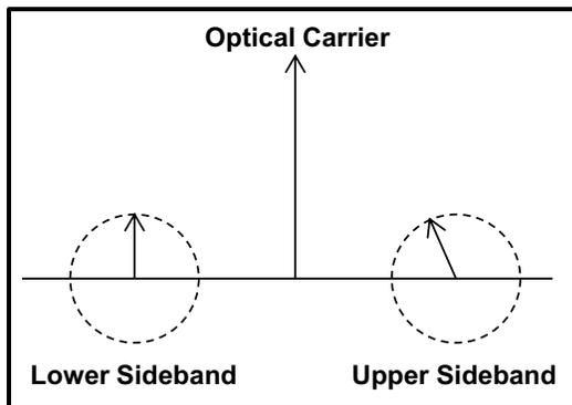
Fig. 8. Chromatic dispersion is the wavelength-dependent propagation velocity in fiber cable.
